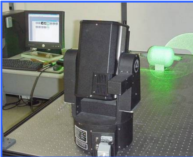
Laser Shearography Set Up for COPV Test
