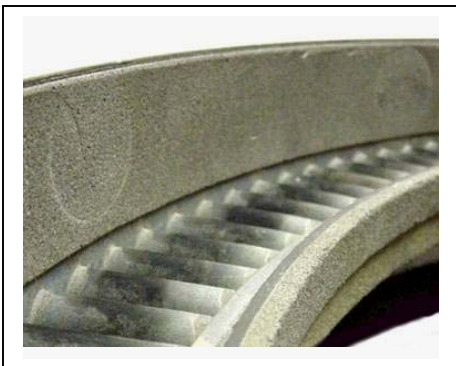
Several examples of turbine engine abrasible seals.
