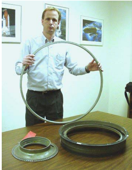
Several examples of turbine engine abrasible seals.
