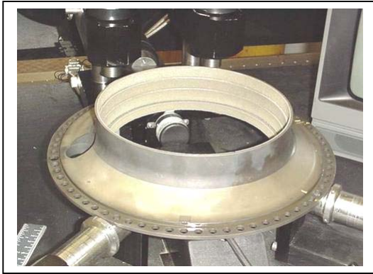
F100 Bearing Seal on test fixture with motorized Rollers and Piezoelectric
