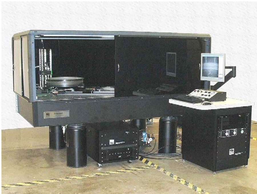
Photo 1 Laser Technology Inc.'s DH-8000 Holographic Inspection Station. The system is composed of 3 sections, the Inspection Station (table, enclosure, and camera), the Control Console Assembly (front right), and the Excitation Assembly (located under table).
