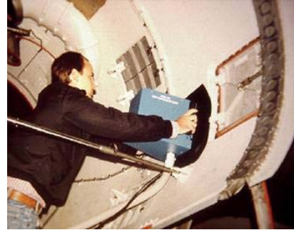
Fig. 2 Typical portable shearography system with built in laser and vacuum window
