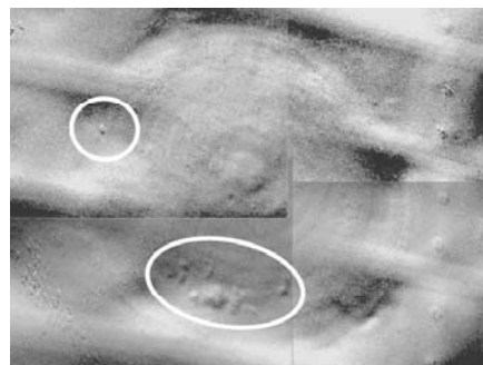
Fig. 3 Shearography image of engineered repair to a solid laminate aircraft structure with far side bonded stringers. Porosity is circled.
