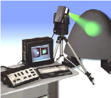
Fig. 1 Typical shearography camera system with built in laser, image processor and controls.
