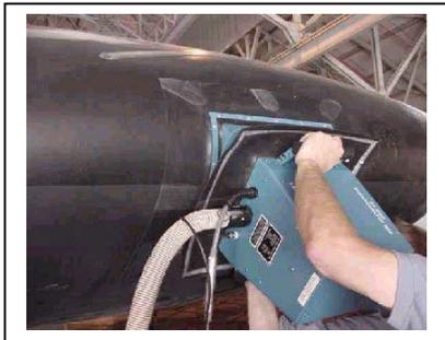
**Figure 3** LTI 4200 Vacuum Hood System rugged design for aerospace and marine composite inspection testing an AWAC E3D radome.
