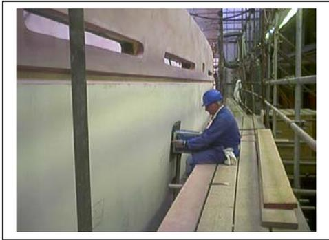
**Figure 6** Up to 10 sq meters per hour at 100% coverage can be achieved. Disbond indications are marked onto the hull surface.
