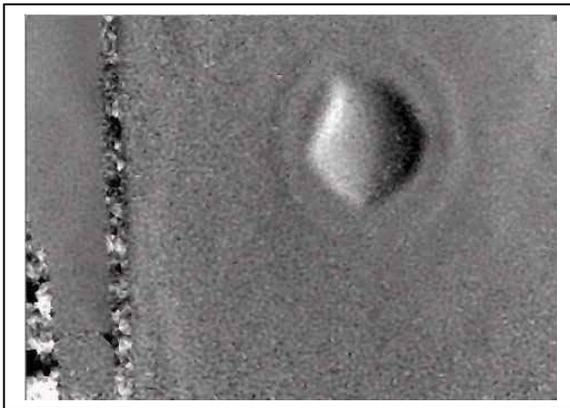
**Figure 10** Programmed disbond detected within a FRP/Foam sandwich, Notice the concentric circle of stronger material (extra bond line) from a sealing cap.
