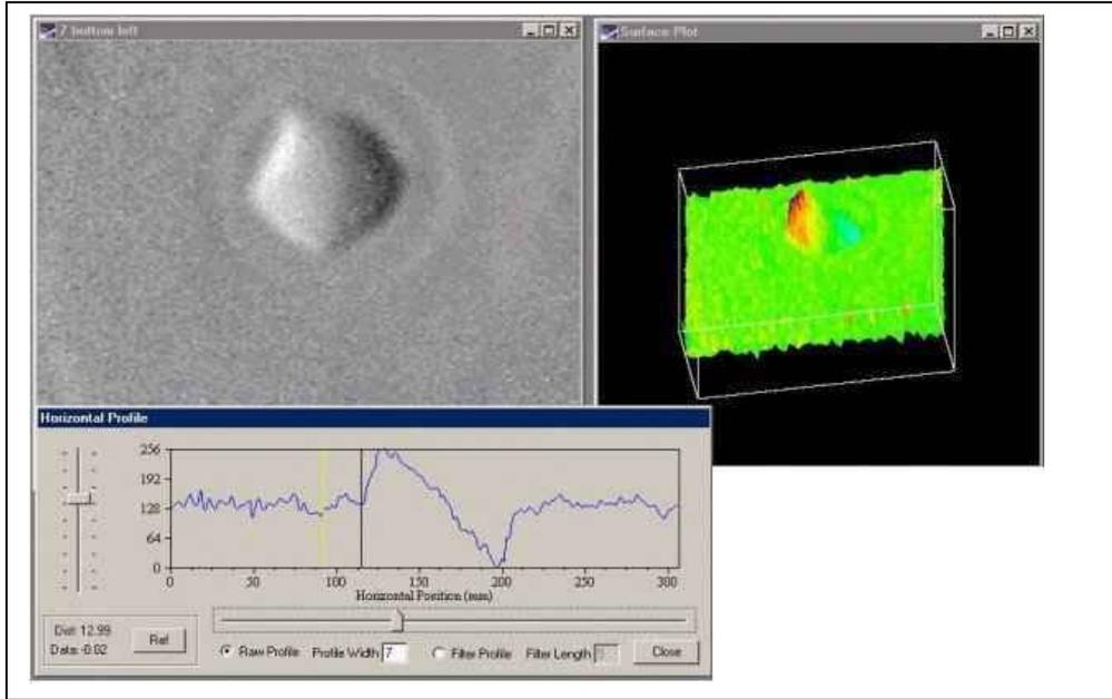
**Figure 11** Shearography Analysis of programmed disbond showing the 3D image and the unwrapped profile of the 1<sup>st</sup> differential of out of plane displacement.
