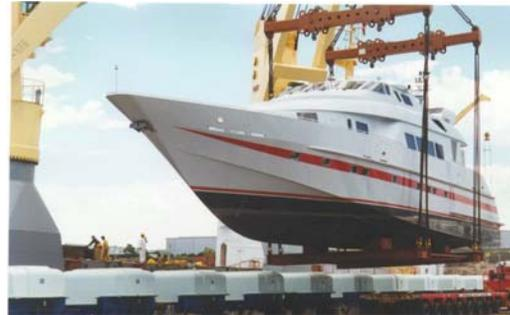
**Figure 2** The 47 meter cruiser MY 'Teeth' inspected by 100% coverage using Laser Shearography during servicing / refit.
