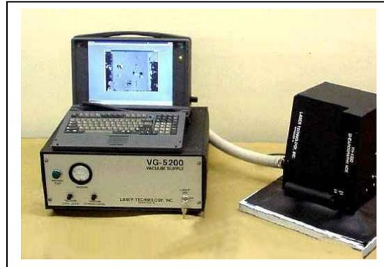
**Figure 5** LTI 5200 Phase Stepping vacuum hood system for enhanced sensitivity.
