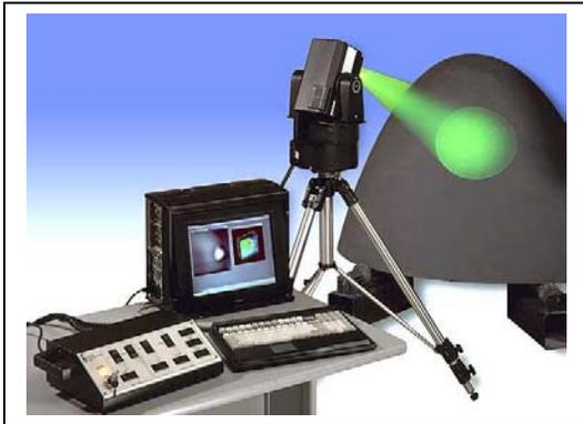
**Figure 4** LTI 5100 Free standing Phase Stepping Laser Shearography camera.
