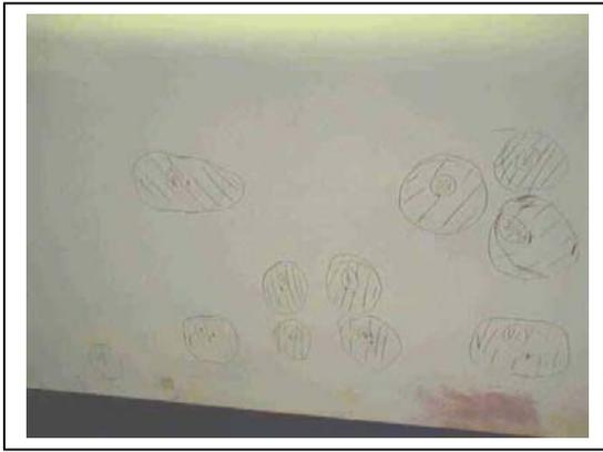
**Figure 9A** Disbond indications marked on the boat hull.
