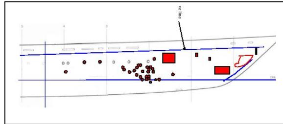
**Figure 9B** Disbond indications mapped on the boat drawing
