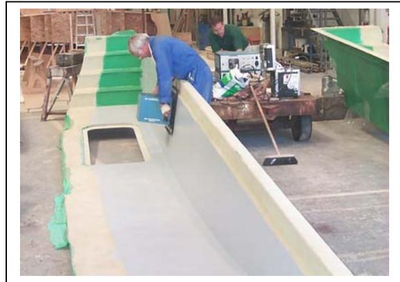
**Figure 8** Example of in process manufacturing Laser Shearography inspection
