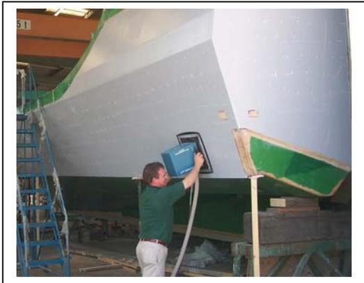
**Figure 7** Example of a Laser Shearography vacuum hood attached during hull inspection
