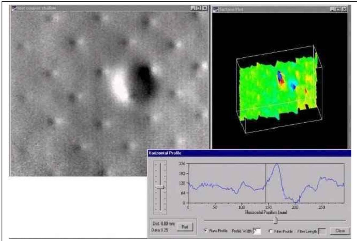
**Figure 12** Breather holes full of core bond clearly stands out under examination – notice they exhibit a 180 degree phase exchange from the programmed weaker disbond, indicating their strength in relation to the weaker disbond.
