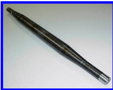
X33 Filament Wound Graphite Strut
