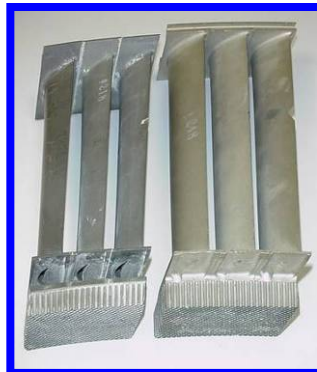
Honeycomb Seals on Stator Vane Clusters
