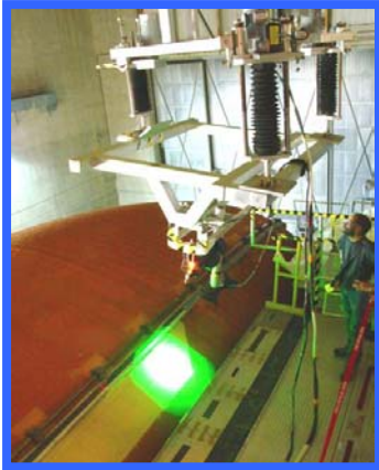
Shearography Camera, LTI-5100 and Exciter mounted to an overhead crane.
