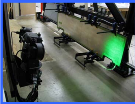
Shearography Camera & Equipped with Thermal and Pressurization excitation on the X/Y 12' high x 20' long Shearography Gantry
